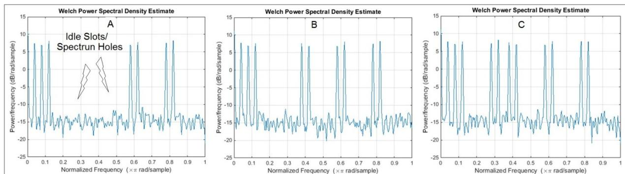
**Fig. 6.** Welch curves showing channel allocation to SUs for QAM signal in AWGN channel for multiple slots. A: 3 PU, 0SU; B: 3PU, 1 SU; C: 3PU, 2SU.
