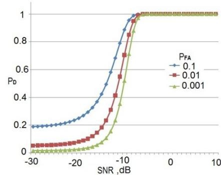
**Fig. 4.** Probability of detection vs SNR at different  $P_{FA}$ .
