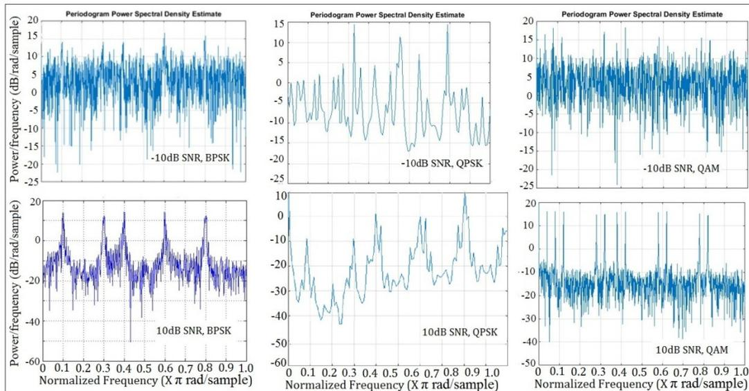
**Fig. 5.** Energy detector output as periodogram psd estimates at SNR -10 db (upper row) and +10 db (lower row) for BPSK, QPSK and QAM signals.
